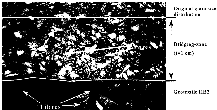
Figure 7. Microstructure at the interface Geotextile HB2/ Soil A (2 nd Test series; hydraulic gradient i=12 )
